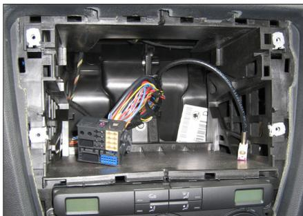
3. Place mounting frame on the dashboard and fix it with the original screws.
