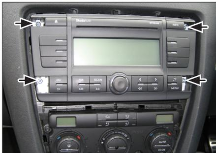
2. Remove 4 screws fixing the OEM head unit.
