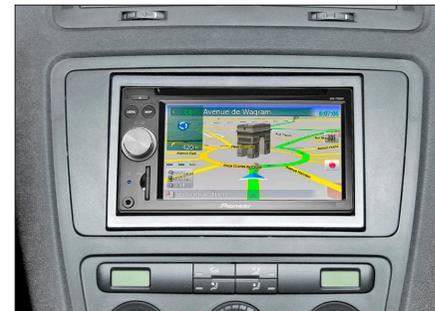
4. Connect all required circuit points and push the double DIN head unit in the metal frame until it snaps in.
