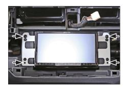
8. Connect all required circuit points and mount head unit on dash board using the 4 OEM screwes removed in step (3)
