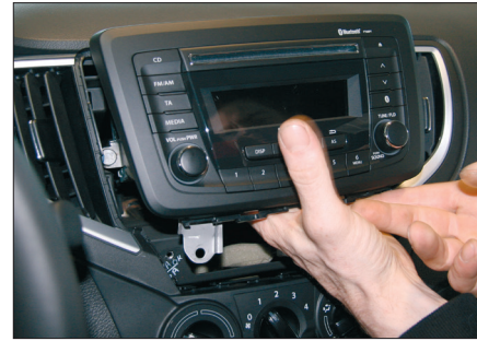
6. Unplug all cables Remove OEM head unit
