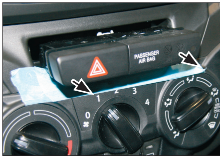
3. Remove plugs - remove switches by pulling them towards your direction
