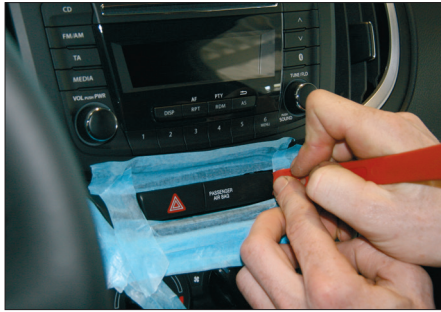
2. Use masking tape in order to protect the surface from scratches. (see photo)
